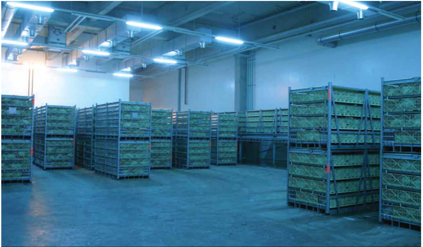
European type Lairage, utilizing blue light to keep the birds calm
